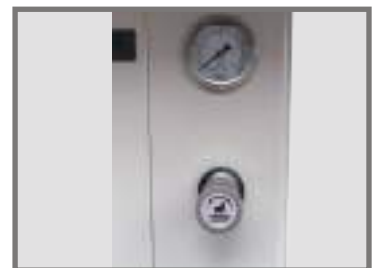
▲ Adjustable clamp pressure
