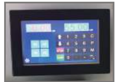
▲ 99 programs with 99 steps each repeat cut function and push out function, touch screen
