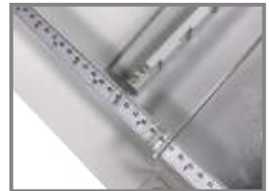
▲ Measuring scale in mm/inch (430M/480M)
